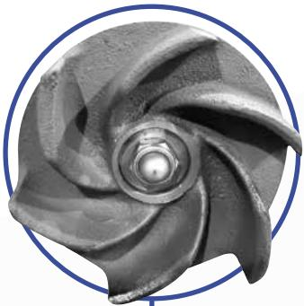
The anti-clogging semi vortex impeller of the DVS allows the pumping **foreign bodies with dimensions up to 70%** of the outlet diameter of the outlet opening
