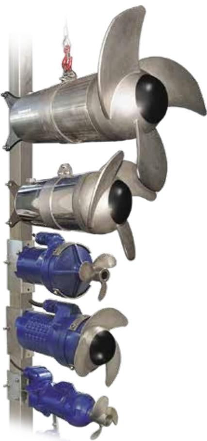
Furthermore, **EBAMIX**, submersed mixers, complete the range. These **mixers** are used for the mixing, homogenization and agitation of heavy sludge and liquids containing solid particles and for the removal of background deposits.
