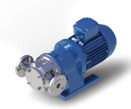
The SVM series are a range of Rotary Vane Seal-less Magdrive pumps that are ideally suited for low flow / high head applications. SVM pumps feature self-compensating sliding-vanes which maintain design head and flow capacities for extended operating life. SVM vane pumps are suitable for thin non-lubricating liquids and/or high differential pressure without rapid wear associated with gear mechanisms.
